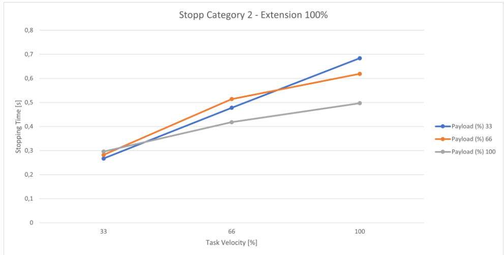
Fig. 17.35: Time; Stopp Cat 2; Joint 2 100%
